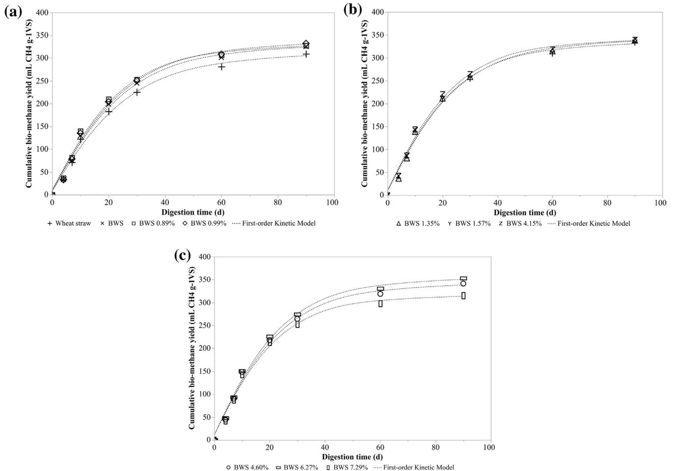
**Fig. 1.** First-order Kinetic plots of cumulative bio-methane yield of wheat straw and briquetted wheat straw (BWS) with KOH injection.
