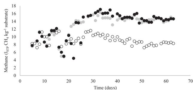
**Fig. 2 – Volumetric methane yield obtained in the lab-scale CSTR from cattle manure (○), cattle manure + shredded wheat straw (●) and cattle manure + briquetted wheat straw (●).**
