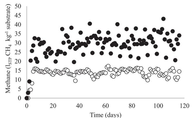
**Fig. 3 – Volumetric methane yield obtained in full-scale CSTR from cattle manure (○) and cattle manure and briquetted wheat straw (●).**
