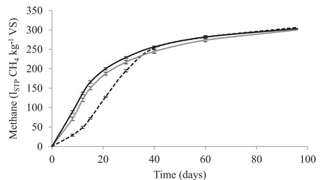
**Fig. 1 – Cumulative methane yield from cattle manure (dotted line), shredded wheat straw (grey line) and briquetted wheat straw (black line) during the batch assay. Error bars: standard deviations.**
